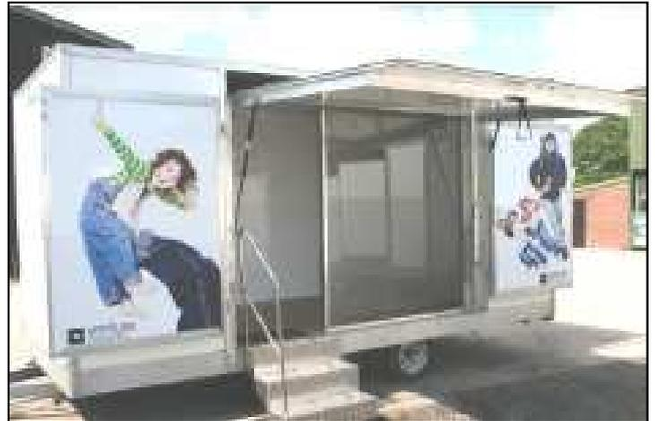
**T43** – One of a group of newly designed trailers that are basic in their application. The walls are not covered in any material to attach graphics with Velcro, but loop and hook tape or Blu-Tack can be used. The units do not have a separate kitchen but we can supply a stand alone unit if required at extra cost. Oak effect vinyl floor with simple clip on steps. No skirting available.
